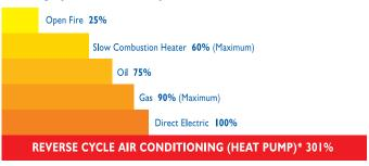
\*Heat Pump heating output is reduced below 5°C outdoor ambient.
