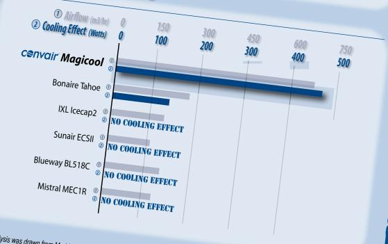
The above analysis was drawn from Meridian Test Laboratory test analysis. The testing was performed by a NATA accredited laboratory to the requirements of Australian Standards AS2913 "Evaporative Airconditioning Equipment". Cooling effect calculated with ambient conditions 38°C DB, 21°C WB, target room
